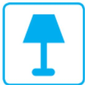
This luminaire contains built-in LED lamps.
